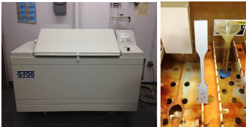
Fig. H-20. Slat fog apparatus (Left image) GFRP specimen exposed to salt fog (Right image)
