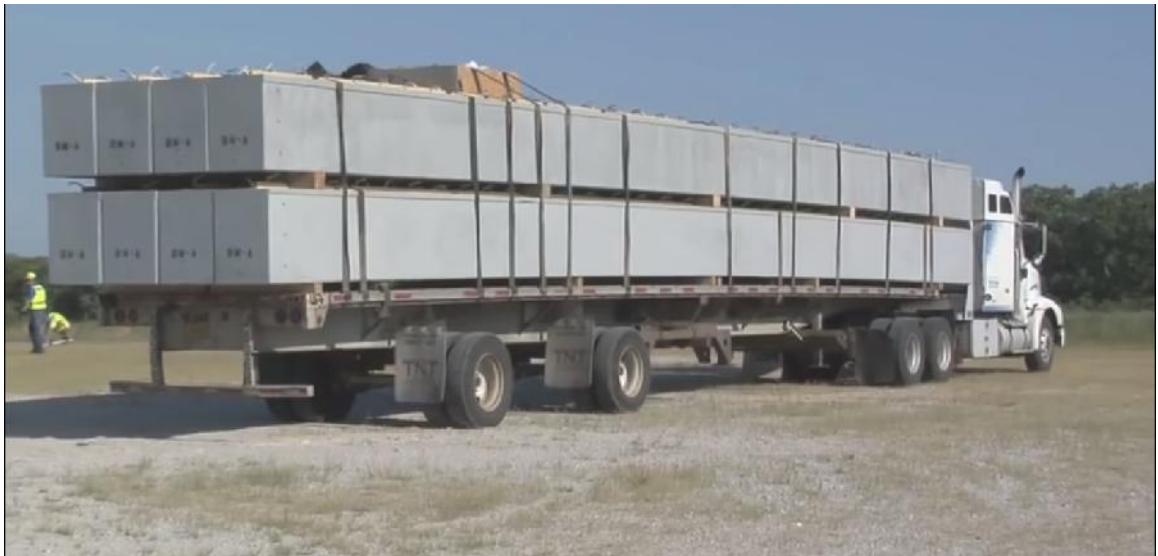
Figure 1.6. Transportation of eight B0439 HCBs with one truck
