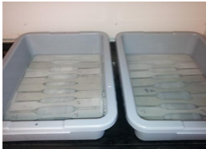
Fig. H-15. GFRP specimens immersed in Alkaline Solution with pH = 13.25
