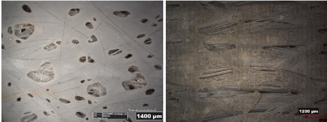
Fig. 15. Optical Microscope images illustrate existing voids at: outer surface (left image) and inner surface (right image) of control specimens
