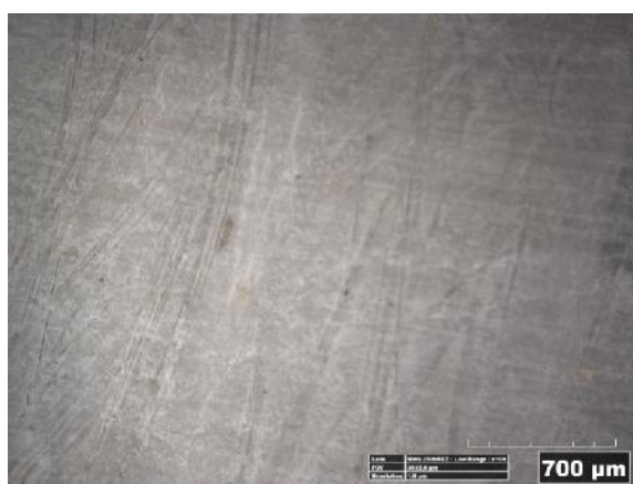
Fig. H-43. No cracks were formed in a specimen (1T-EC-LW) exposed to thermal cycles in the environmental chamber
